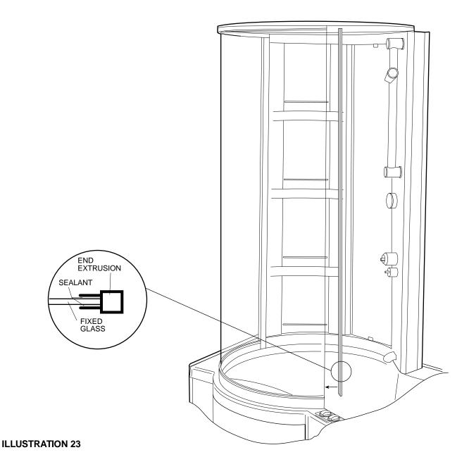
13. Apply sealant in frame and extrusion. Align and place extrusion above end cap onto the fixed glass.
